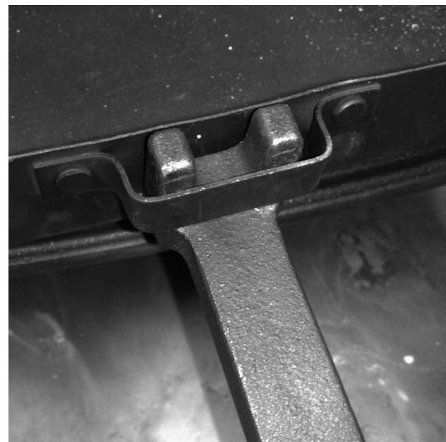
The forked end of the tool is inserted underneath the ash pan grip as shown above to create the ash pan handle.
